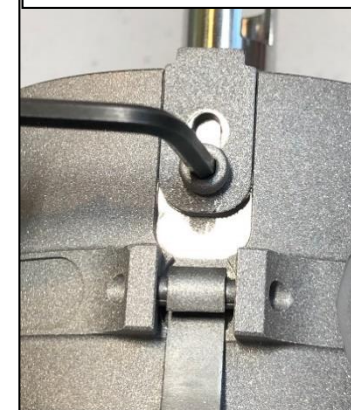
Cap Index Slide for changing between Brown and Black Cap.
