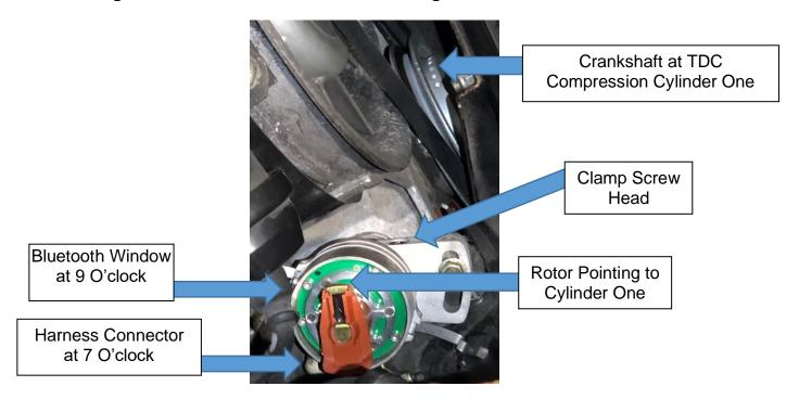
5. Rotate the rotor in the distributor so that the rotor is pointing to slightly CCW of the same location as the old distributor when it was removed. Then push the distributor all the way into the engine
