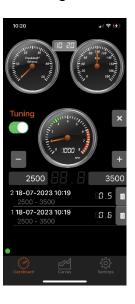
The X button closes the page and returns to the dashboard page. The – and + buttons adjust the mechanical timing one degree at a time.
