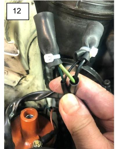
**NOTE: You may elect to cut the loop terminals off and use a marine type wire splice instead of using the loop and bolt terminals.**
