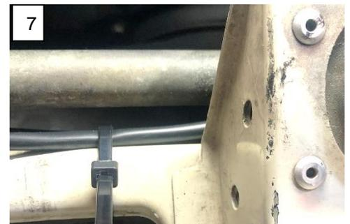
**CAUTION: Failure to route the harness clear of the moving parts can cause damage to the harness, radiator fans and or headlight mechanism.**
