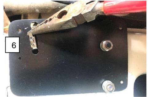
4. Thread the Cube module harness wires between the notch on the bracket and the headlight actuator lever placing the module on the bracket. Secure the module to the bracket by screwing the three sheet metal screws into the pilot holes of the bracket as shown in picture 6.
