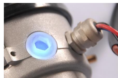
Low Voltage Tachometer connection for points type tachometers.
