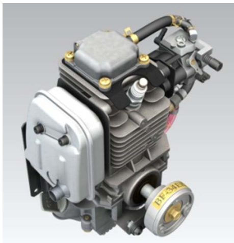
Figure 10 CAD model of Fuji Imvac-34EI engine modeled by one of the undergraduates.
